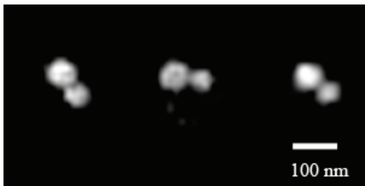
Figure 6-6: Scanning electron microscope images of GNP 80 and GNP 40 hybridisation pairs. The images were acquired using a Philips XL30 eSEM in environmental mode at 15 KV at 10,000× after sample drying under a flow of nitrogen gas.
